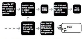
NB. The factory default settings for the 2nd ON/OFF times are both set at 12:00pm (midday) which cancels this 'ON' period giving 2 ON/OFF periods for 24hrs. If a midday 'ON' period is required set the 2nd ON and OFF times accordingly. If not press ENTER twice.
